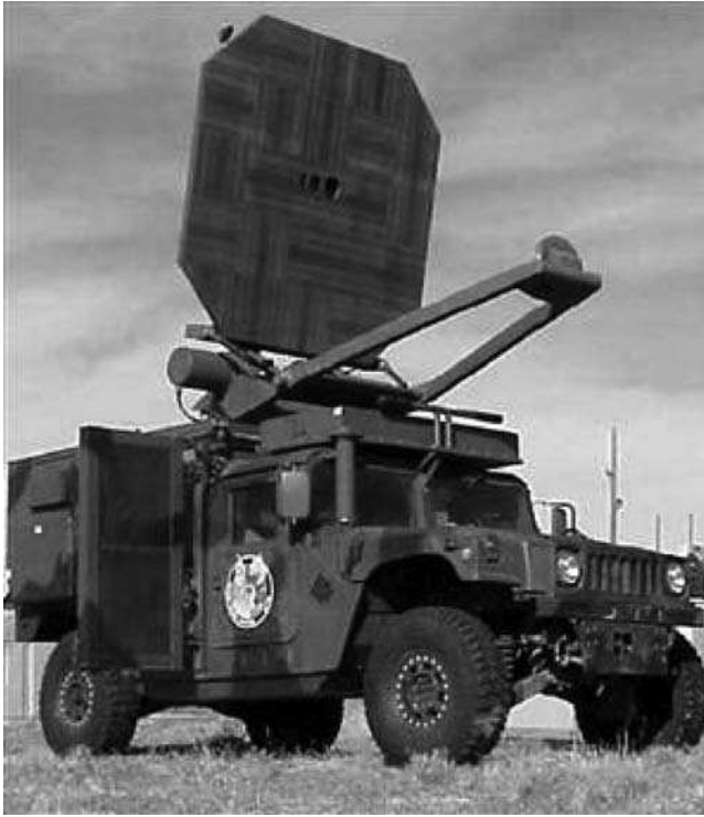
FIGURE 3.6 Active Denial System, a nonlethal microwave weapon.
